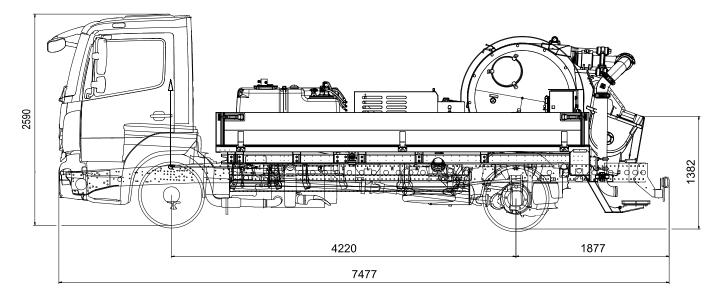
Note: Standard version. Dimensions and weights depend on truck, pump model and equipment. Dimensions in mm. For illustration only.
